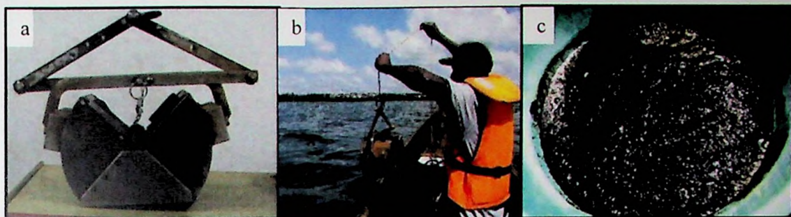
Plate 3.3: Collection of sediment samples using a sediment ponar grab
