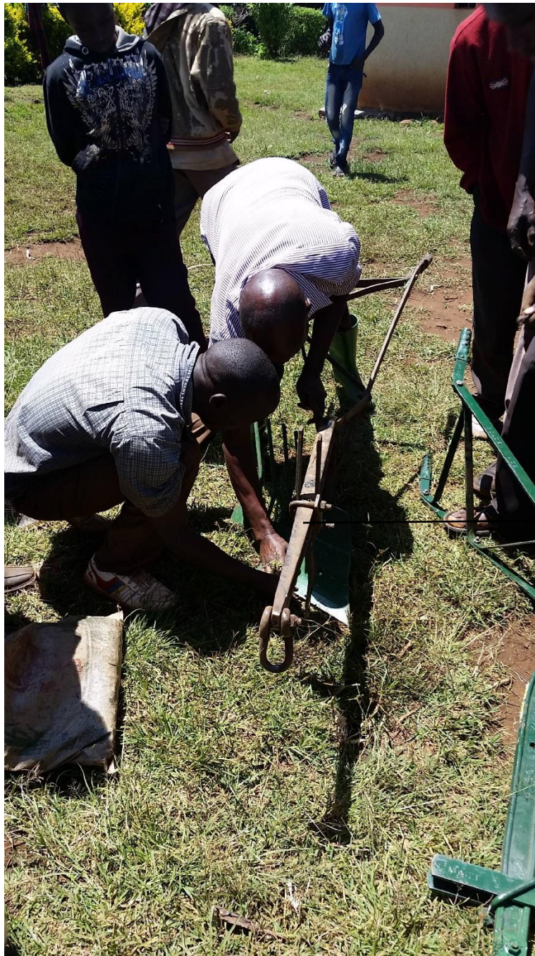
Figure 5: Innovative farmer transferring forked/pronged attachment onto Sebei frame which has a much shorter beam and share than ordinary plough frame (brown frame) with pronged end (green) replacing the mouldboard
